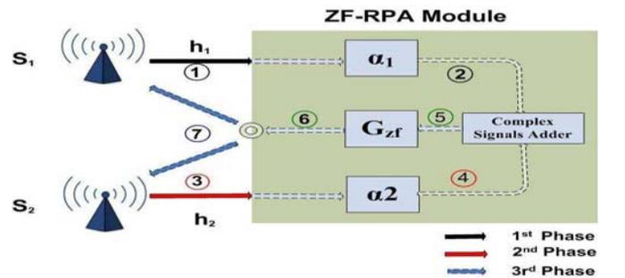
Fig. 2: Block Diagram of ZF-RPA Module with TDBC protocol.
