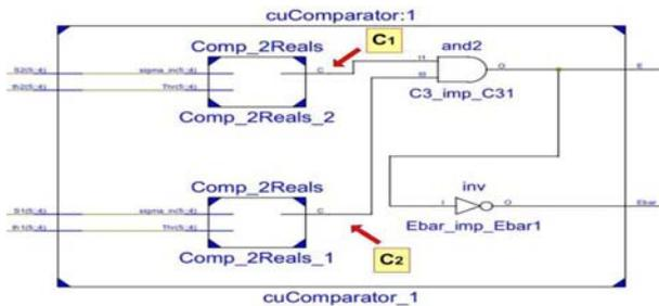
Fig. 6: RTL Schematic of the Fixed-Point Comparator.
