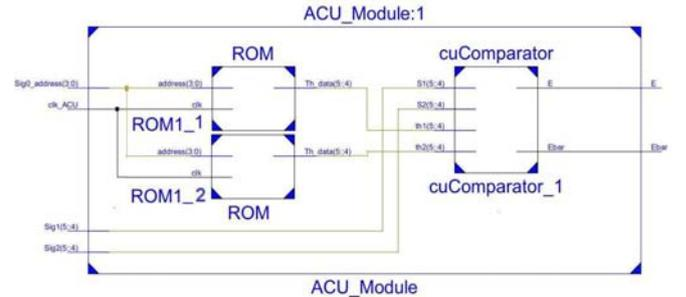
Fig. 5: RTL schematic of the ACU.
